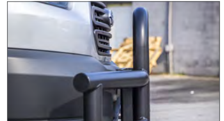
3" diameter, 14-gauge stainless steel tube design for added vehicle protection
