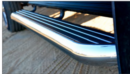
Extruded aluminum core to be strong, lightweight and rust-free
