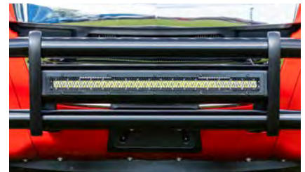
IP68 and IP69K waterproof and dustproof ratings keep water and air from getting inside
