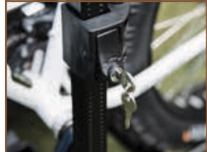
Lockable, ratcheting arms will not loosen during travel
