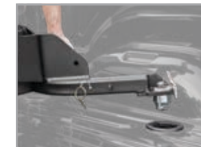
Step 1 - Drop the legs into the truck bed puck system
