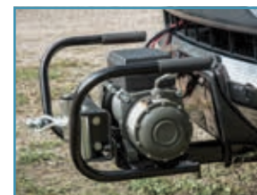
Winch mount for convenient hitch attachment as needed
