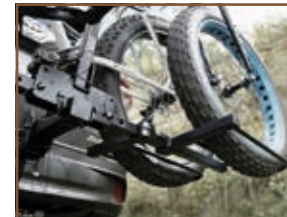
Replacement cradles available to fit fat tires up to 4-7/8" wide
