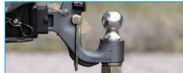
Cupped hook tightly holds lunette ring fore and aft to reduce chucking and noise
