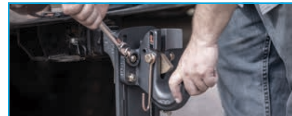
Slotted bolt plate for quick, easy, one-tool height adjustments – no disassembly required
