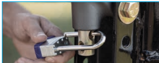
Drop-in pin accepts lock to deter theft (turns 90 degrees while coupled)
