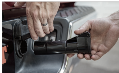
Insert Echo ® between the vehicle-trailer 7-way RV blade connectors
