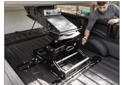
Automatically latches in both directions so you only have to exit the truck once
