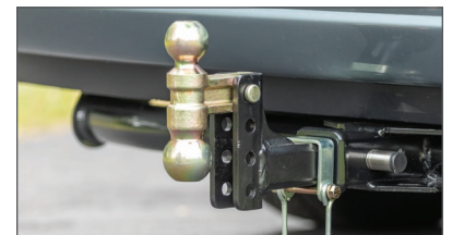
One-pin dual ball attachment for quick, easy adjustment
