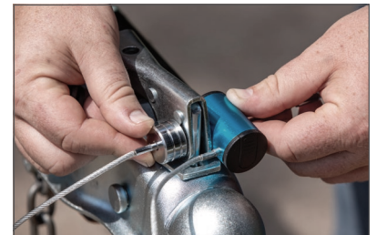
Lasso lock can be used to lock the coupler latch while towing
