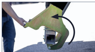
Pivoting, fold-out design positions the stepping surface behind the trailer
