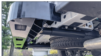
Designed to absorb rear impacts up to 5mph and avoid possible frame damage
