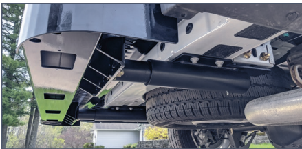
Spring-loaded shock-absorbers built into the mounting brackets
