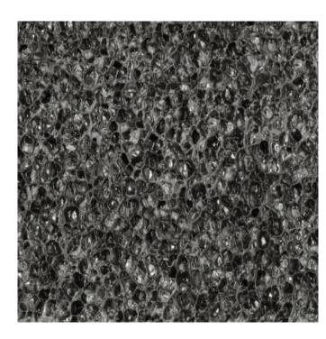
Cross-linked polyethylene foam adds comfort and helps limit road noise
