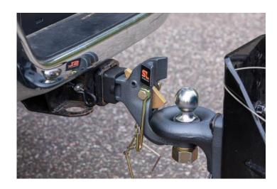
**Auto-lock**: The auto-locking latch will engage without the need for manual coupling. Just insert the safety pin!
