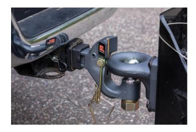
**Drop**: With the lunette ring centered on the pintle hook, drop the ring down onto the hook by lowering the trailer jack.
