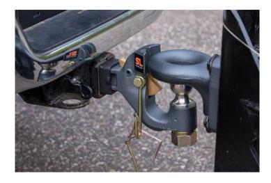
**Strike**: Back up your vehicle to the trailer. An integrated strike plate on the pintle hitch helps stop and center the lunette ring.
