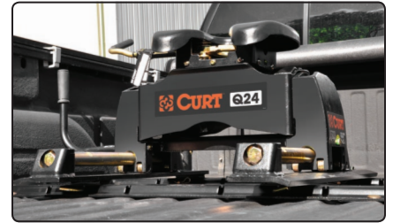
16570 R24 roller shown installed in a truck bed with 16545 Q24 head unit (16546 kit)
