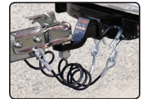
Safety cables in use
