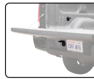
Route 7-way socket into truck bed
