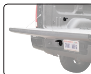
Route 7-way socket into truck bed (7')
