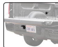
Route 7-way socket into truck bed (10')
