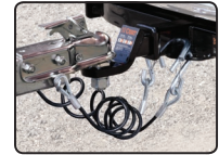
Safety cables in use
