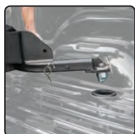
Step 1 - Drop legs into the truck bed's anchoring system
