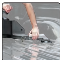
Step 2 - Close the anchor levers to lock legs into place
