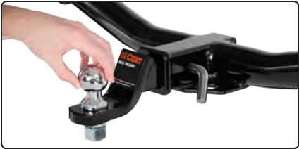
Twist the ball down onto the shank to lock
