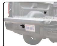
Route 7-way socket into truck bed (10')
