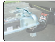
25035 securing a coupler latch
