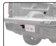
Route 7-way socket into truck bed (10')
