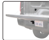
Route 7-way socket into truck bed (7')
