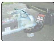
25035 securing a coupler latch
