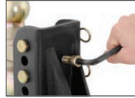
Built-in anti-rattle prevents shaking (45901 and 45902)
