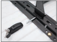
Locks a 5th wheel to industry-standard rails
