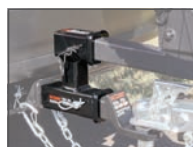
45792 provides two receiver tubes
