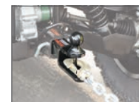
Clevis pin accepts hook or strap for straight-line pull
