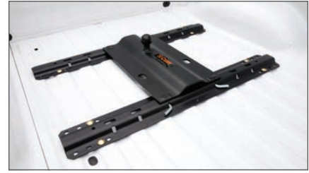
C Using pre-existing 5th wheel base rails
