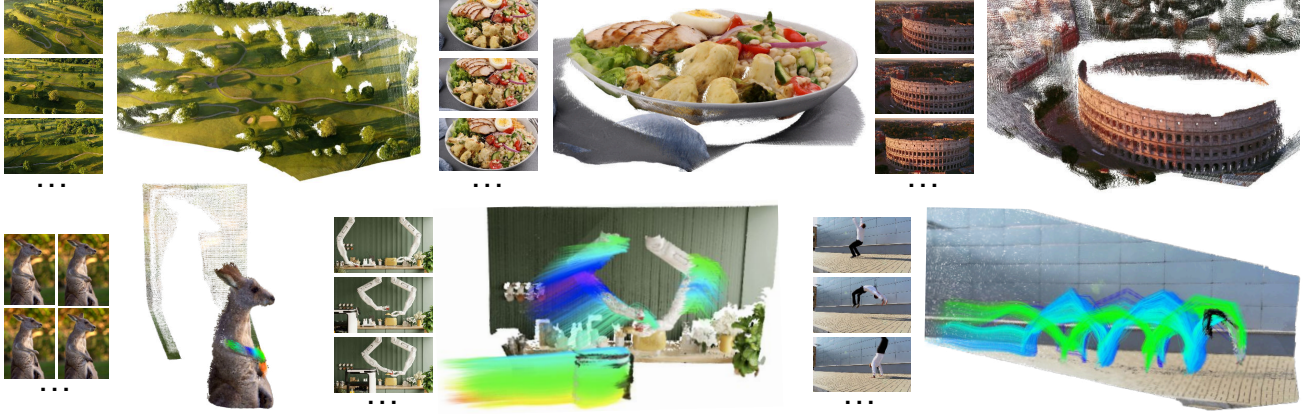
Figure 5. Visualizations on in-the-wild videos – D4RT demonstrates accurate reconstructions on static (top row) and dynamic scenes (bottom row). In the presence of motion, D4RT additionally produces robust 3D point trajectories.
