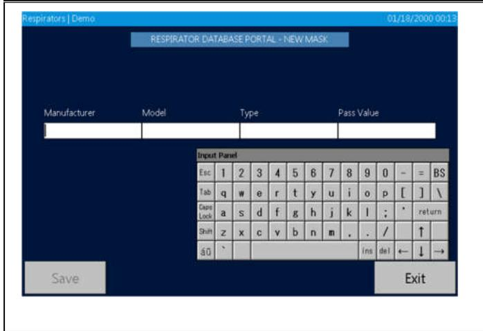
Enter information into the [Manufacturer], [Model], [Type], [Pass Value] fields, and tap the [Save] button to confirm the entry.
