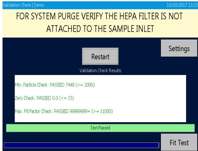
To confirm whether the device performs correctly, this test confirms the fit factor using the HEPA filter. The instrument measures the particle concentration in the ambient air and calculates the ratio to the particle concentration via the HEPA Filter. By determining this ratio, the device confirms that it is correctly performing this function.
