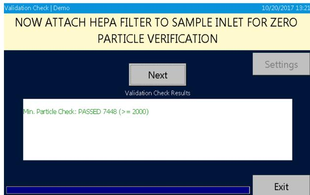
If a leak occurs inside of the device, the test result may be affected. The Zero Check determines that there are no internal leaks or loose connections.
