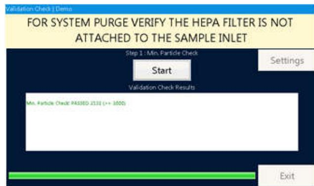
Remove the HEPA filter or the mask if attached, and tap the [Start] button to check that the particle concentration in the ambient air is sufficiently high enough to calculate the mask fit factor. Depending on the ambient particle concentration (i.e., outside of the mask), the environment may be inappropriate to perform a mask fit test. This process also confirms that the device is operating properly. When this measurement is complete, proceed to the Zero Check
