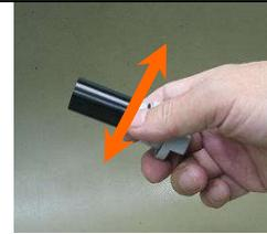
Failure to do this may cause the absorbed alcohol to clog the front of the alcohol cartridge. As a result, the flow of the incoming airborne particles and alcohol vapor will be disturbed, making it impossible to measure correctly.
