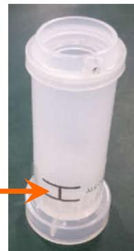
4. Insert the alcohol cartridge into the alcohol storage container, and turn it about 45° clockwise until it is firmly locked. Do not use excessive force.
