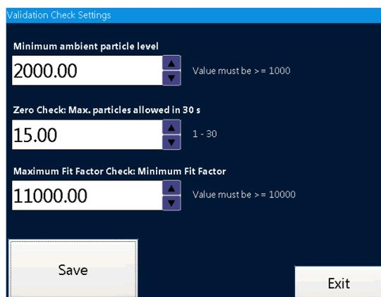
By tapping the [Setting] button on the Validation Check screen, you can change the value(s) for the check as necessary. After changing the value(s), tap the [Save] button to save the change(s).
