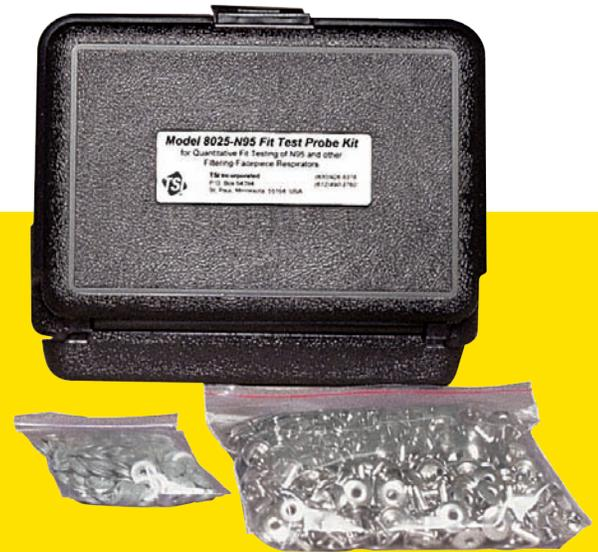
The kit includes 500 lightweight disposable sampling probes and easy to use installation tools. It only takes a few seconds to puncture the mask, insert a probe and then press a push nut on from the other side. The PortaCount Pro+ Fit Tester sample hose fits directly onto the exposed end of the sampling probe.
