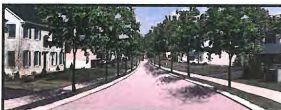
Traditional Neighborhood Design: Narrow streets, smaller building lots & set-backs, and abundant sidewalks & street trees.
