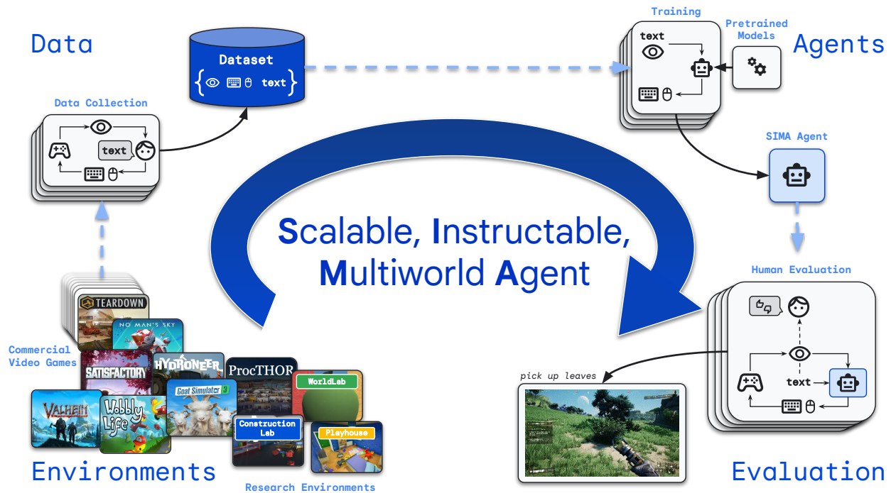
Figure 1 | Overview of SIMA. In SIMA, we collect a large and diverse dataset of gameplay from both curated research environments and commercial video games. This dataset is used to train agents to follow open-ended language instructions via pixel inputs and keyboard-and-mouse action outputs. Agents are then evaluated in terms of their behavior across a broad range of skills.
