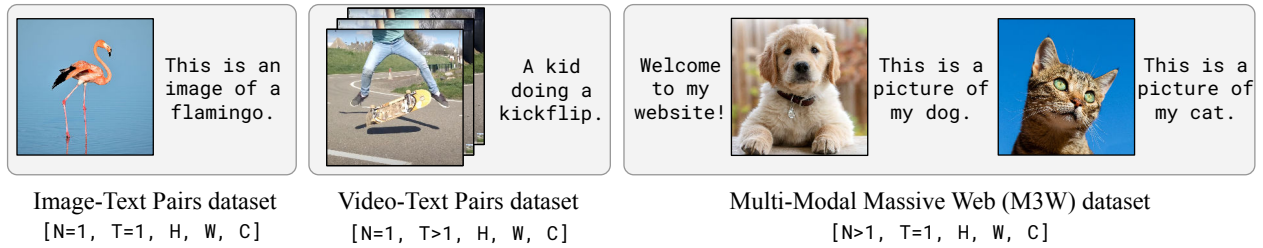
Figure 7 | Training datasets. Mixture of training datasets of different nature. N corresponds to the number of visual inputs for a single example. For paired image (or video) and text datasets, N = 1 . T is the number of video frames with T = 1 being the special case of images. H, W, C are height, width and color channels.
