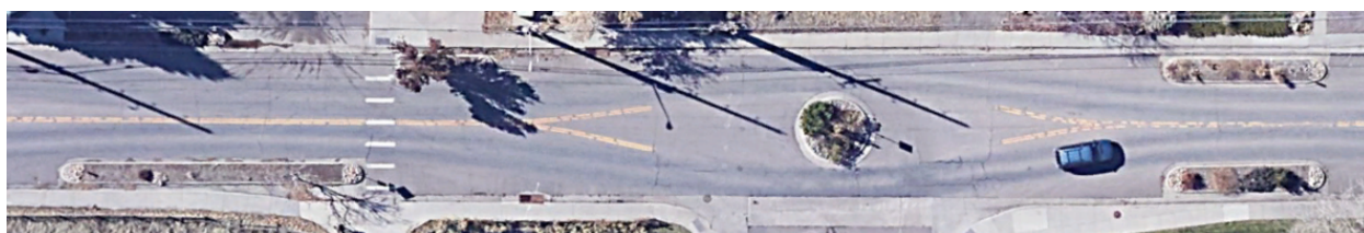
Figure 2: Traffic being rerouted around obstacles to slow speeds on Ford Street in Golden, CO.
