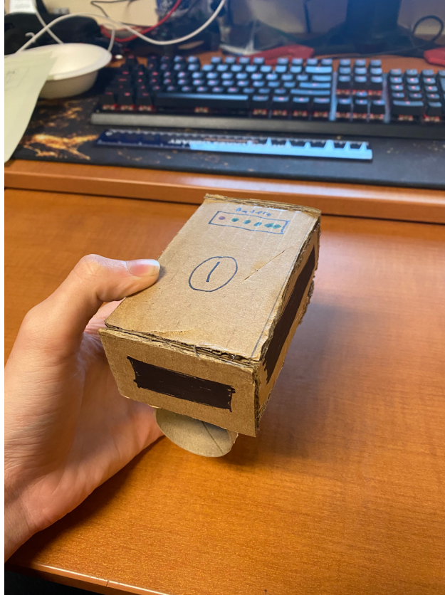
Figure 36: Looks-like prototype for our final design choice. Emitter portion.
