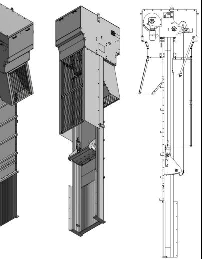
Inclination 90° Channal depth 1 ... 20m Channal width 600 ... 2500mm 10,15,20,25,30, Bar spacing 40,50,60,80,100mm
