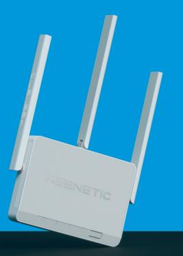
580 MHz MIPS 24KEc CPU; 64 MB DDR2 SDRAM; 16 MB flash memory (Dual Boot); AES 128/256 crypto accelerator.
