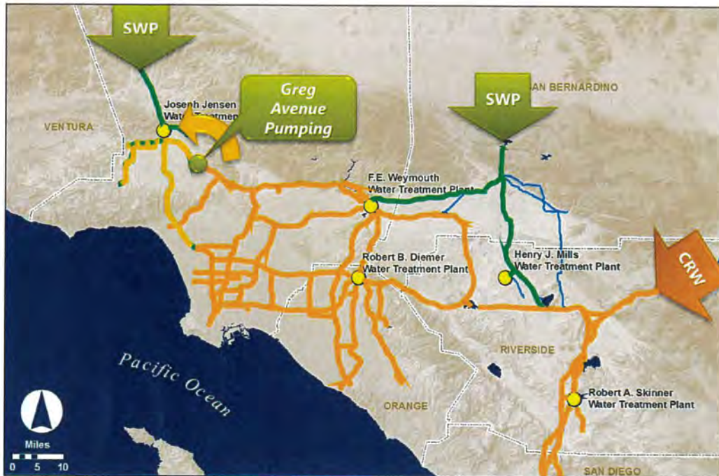
Greg Avenue Pump Station enables delivery of Colorado River water to Calleguas service area http://www.mwdh2o.com/PDFWWACurrentBoardAgendas/05102021%20EO%207-4%20Presentation.pdf
