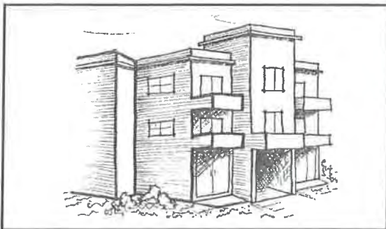
Parapet and cornice in flat roof.
