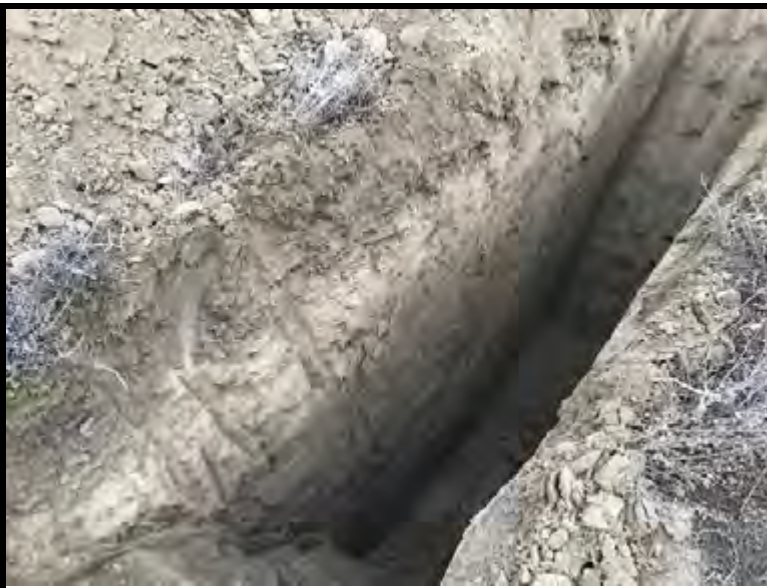
Subsurface soil profile within test pit TP-1
