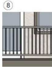
METAL GUARDRAIL PAINTED SW 7042 SHOJI WHITE
