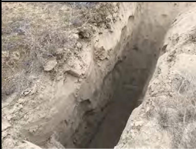
Subsurface soil profile within test pit TP-11
