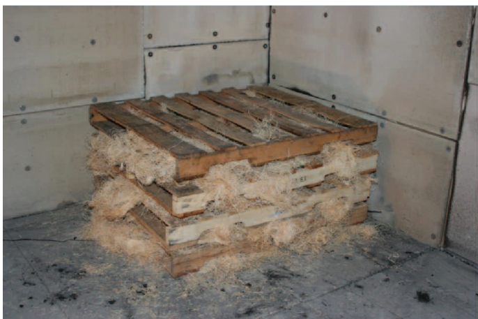
Figure A-3. Fuel and Excelsior Source for Slow (top) and Fast (bottom) Ignition Scenarios
