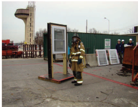
Figure 12: Ground Level Window Breakage Prop
