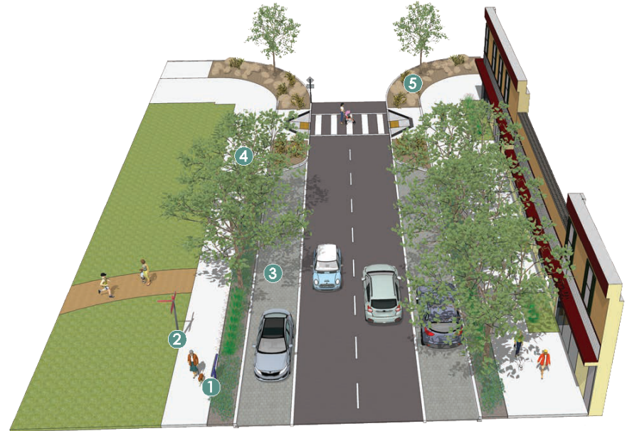
FIGURE T-11: Green Street or Urban Trail Community Corridor (Urban Trail/Green Street)
