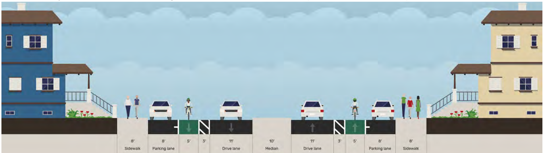
FIGURE 6-6: Bicycle Lanes with Parallel Parking and Painted Buffers on Both Sides (80' ROW, 64' Curb to Curb)
