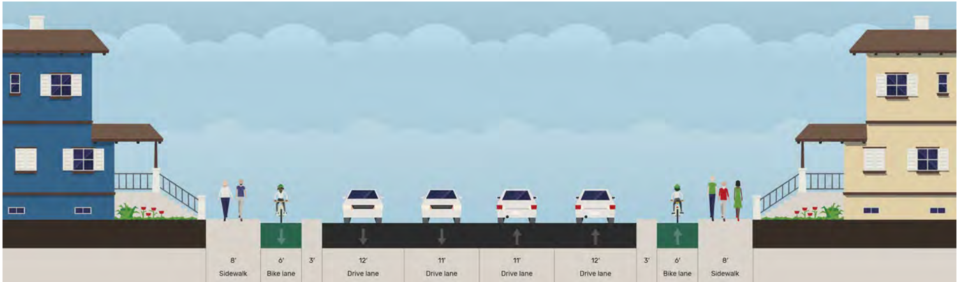
FIGURE 6-5: Bicycle Lanes with Raised Medians on Both Sides (80' ROW, 64' Curb to Curb)
