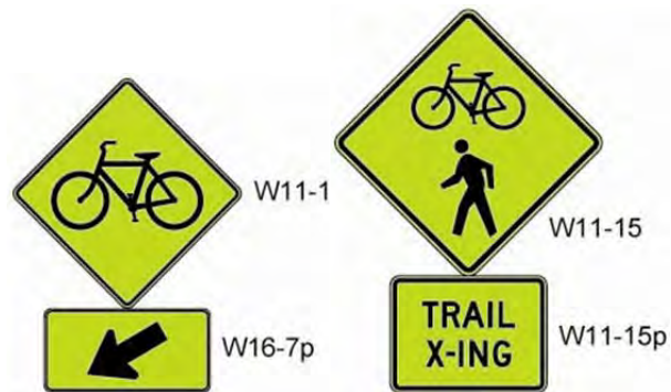
Recommended signage from FHWA-MUTCD, Figure 9B-3
