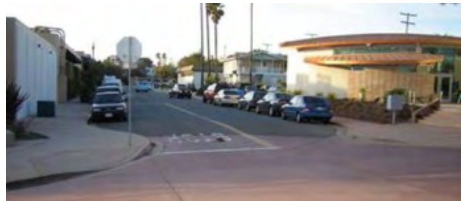
Example of a bulb-out at an intersection
