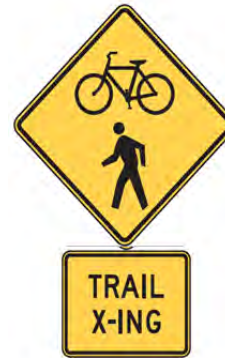
Warning signs are yellow, such as this combination of W11-15 and W11-15P from the MUTCD
