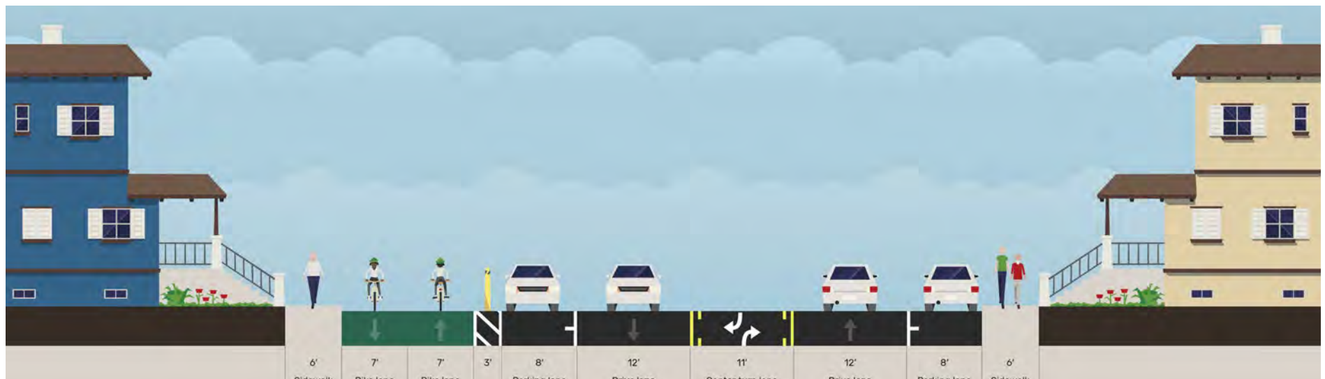
FIGURE 6-16: Bicycle Lanes on One Side with Buffer and Parallel Parking (80' ROW, 68' Curb to Curb)
