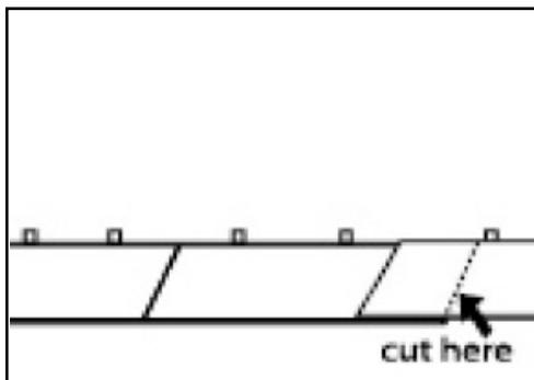
Using a sharp utility knife or shears and a straight edge, score a line on the top surface of the plank. The plank should split on the score line with little effort. Use saw to cut plank to size. Note: the **end pieces must be longer than 8"**. This may require cutting a plank to start a row depending on the size of the room.
