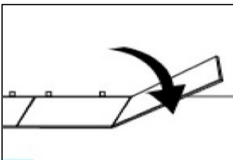
Continue along the wall until you reach the last full plank, connecting each plank in manner described above. To fit the last plank, turn plank over (face down). Place the plank in the corners so the tongue on the short end touches the adjacent wall. Measure overlap between the installed plank and the last plank.
