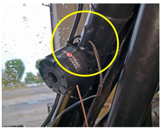
Installed antenna on the Buzzer unit (optional only when using extension cable).
