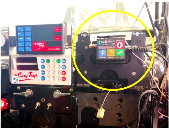
Installation of the Com-Box unit with bracket on the dashboard using bolts.
