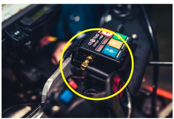
Installed antenna on the Com-Box unit.
