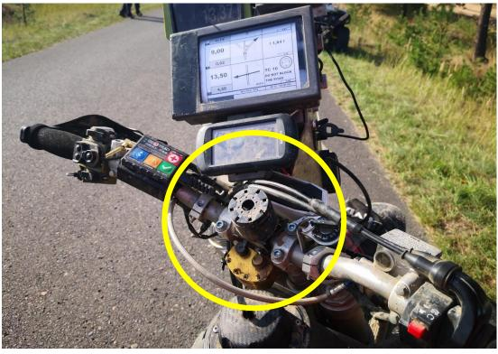
Installation of the Buzzer with bracket on the handle bar using cable ties.
