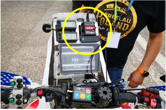
Installation of the GPS TRACKER on the navigation tower using cable ties.
