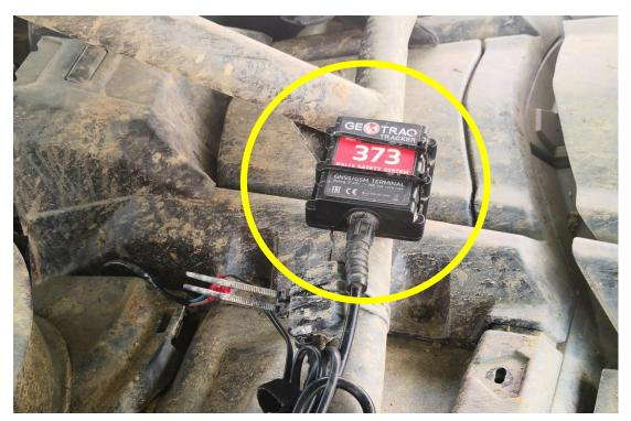
${\it Installation of the GPS TRACKER on the railing of ATV using cable ties.}$
