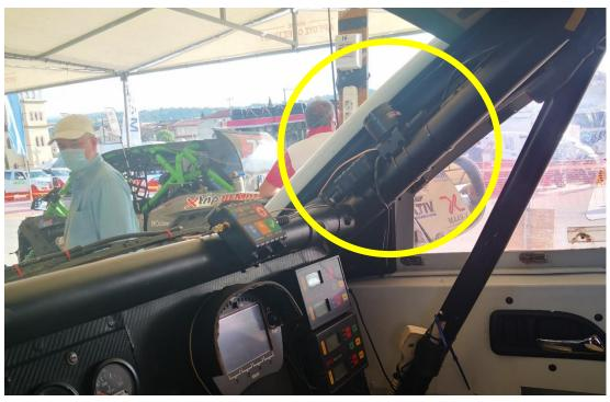
Installation of the Buzzer with bracket on the Roll cage using cable ties.
