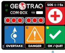
If you receive a SOS signal from Lights will **BLINK RED. ALARM IS ON.** CONFIRM WITH OK/QUIT BUTTON AND BE READY TO ASIST AN ACCIDENT SCENE.
