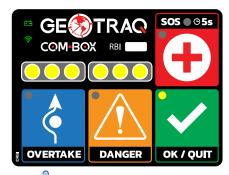
Vehicle A wants to overtake: press for 2 seconds the BLUE BUTTON to send a signal to the vehicle ahead (less than 200m).
