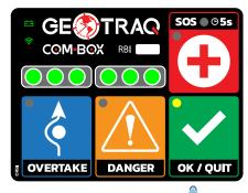
Vehicle A receives confirmation for overtaking: Lights ARE SOLID GREEN, vehicle B will allow overtaking at the first safe place.
