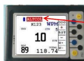
Warns the competitor that another vehicle arrives in the inverse direction unless 200m (+ the buzzer rings).
