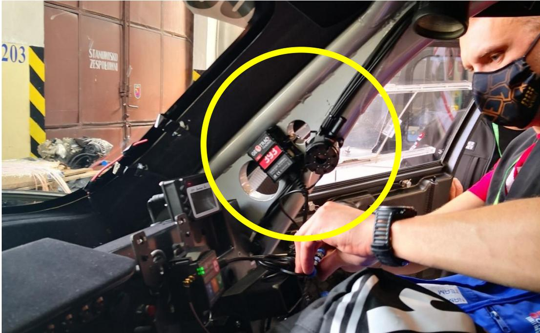
*Installation of the Buzzer with bracket on the Roll cage using cable ties.*
