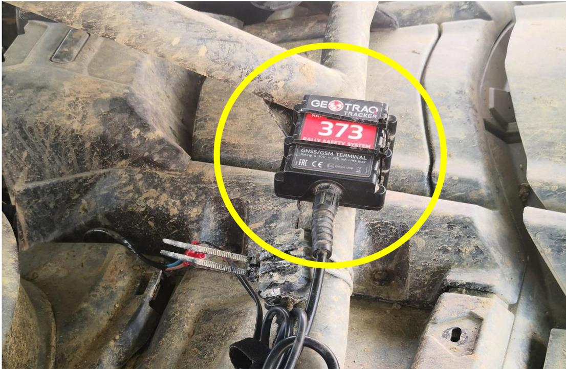
*Installation of the GPS TRACKER on the railing of ATV using cable ties.*
