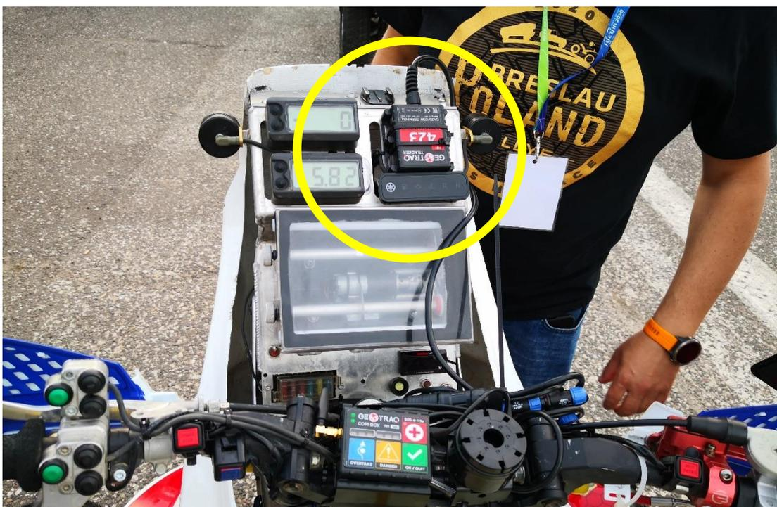
*Installation of the GPS TRACKER on the navigation tower using cable ties.*
