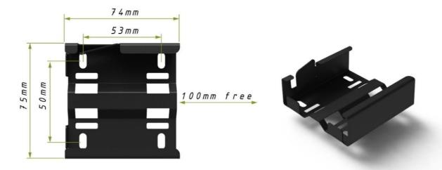
At least 10 cm of space must be left on the sliding side of the Base / Mount bracket to allow the installation of the Com-box.
