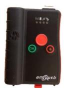
This communication is done in two ways, via voice allowing the RC and the crew to exchange information about the reason for retiring, and the state of the occupants and via the GPRS communication link, the equipment has with the Rally Control.
