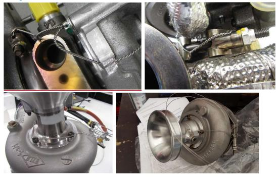
Examples of incorrect sealing wiring
