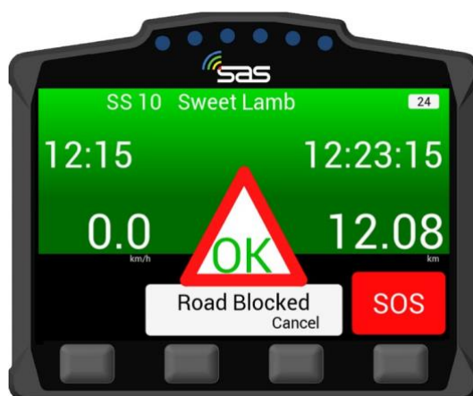
SCREEN 7A. OK – Road Blocked
