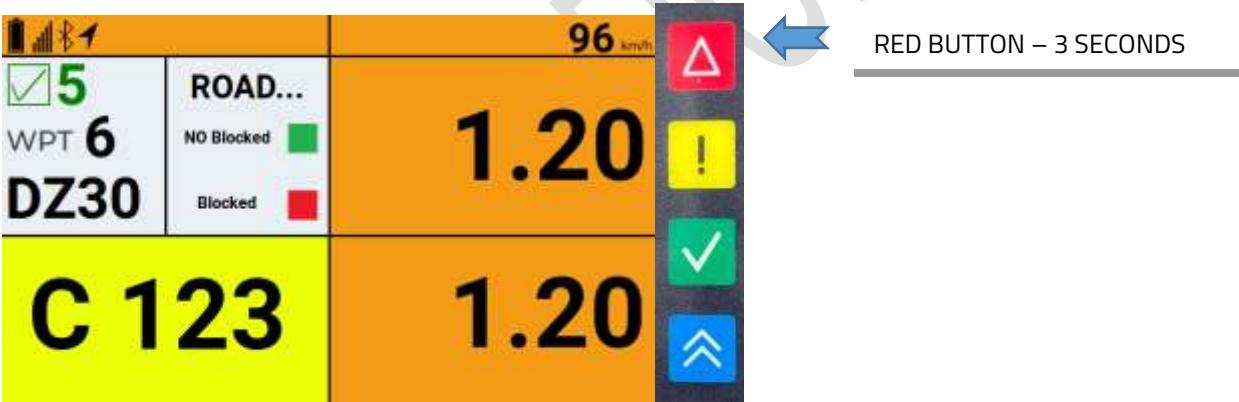
Photo 4. Display BREAKDOWN WARNING – Confirmation Blocked or not.
