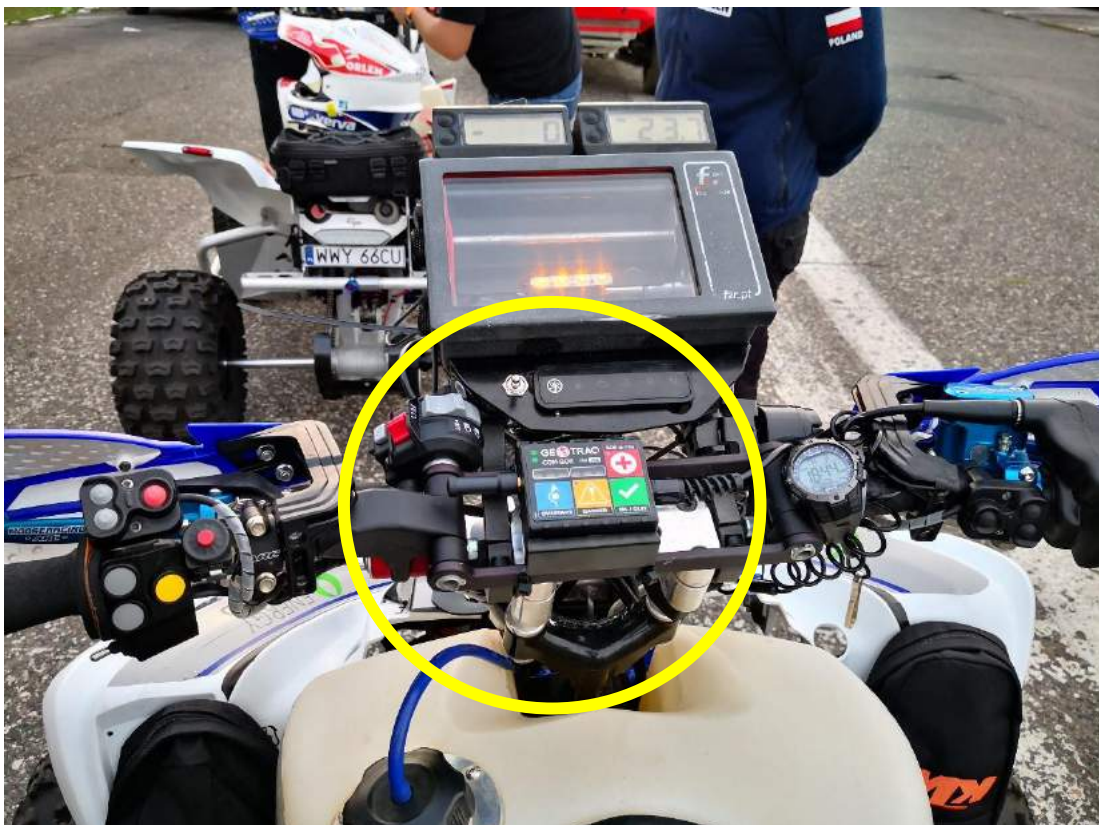
Installation of the Com-Box unit with bracket on the handle bar using cable ties.
