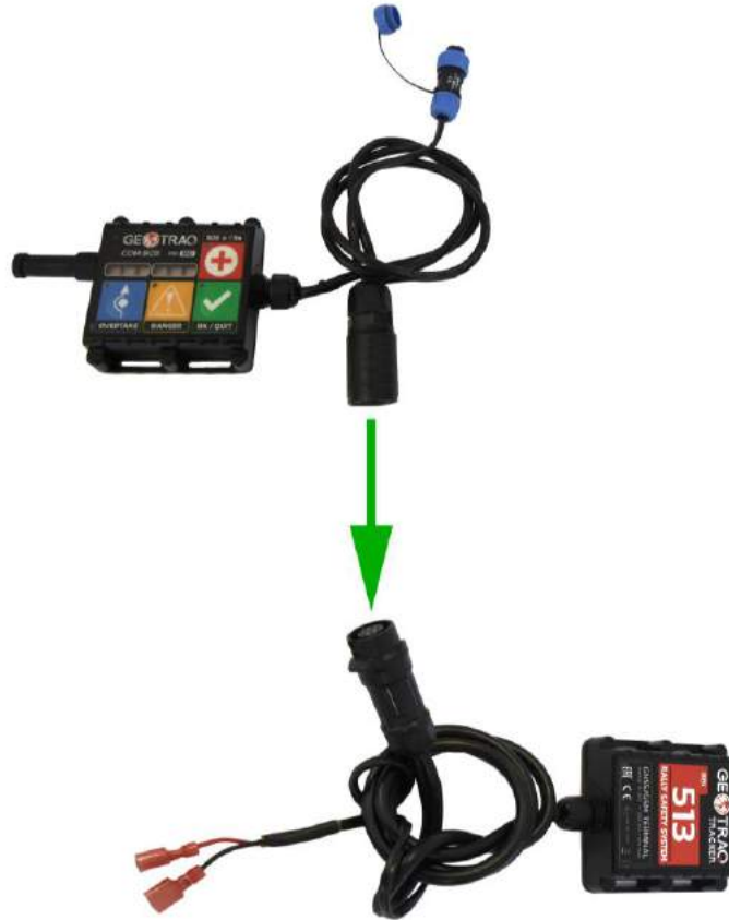
Connect the COM-BOX to the TRACKER.
