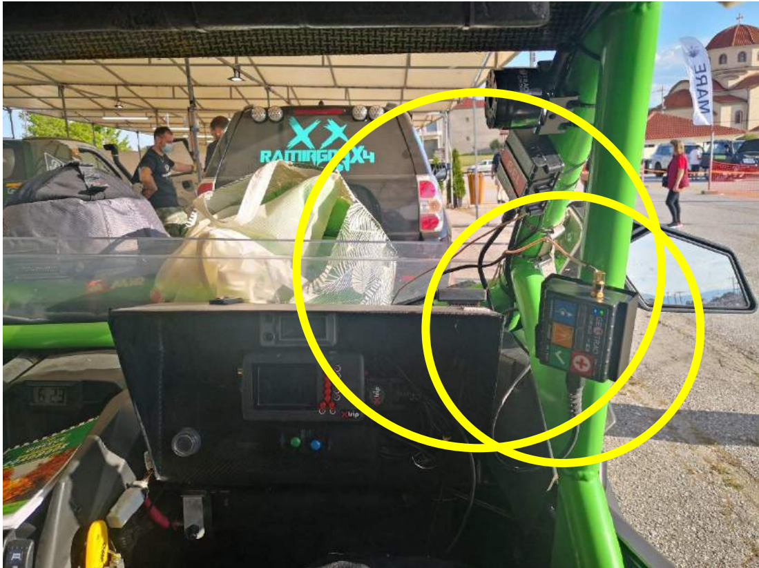
Installation of the Com-Box unit with bracket on the roll cage using cable ties.
