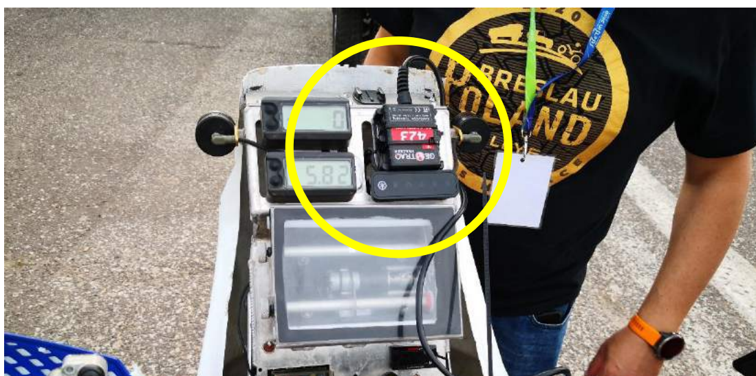
Installation of the GPS TRACKER on the navigation tower using cable ties.
