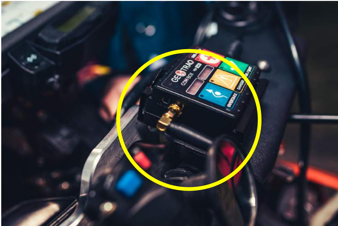
Installed antenna on the Com-Box unit.
