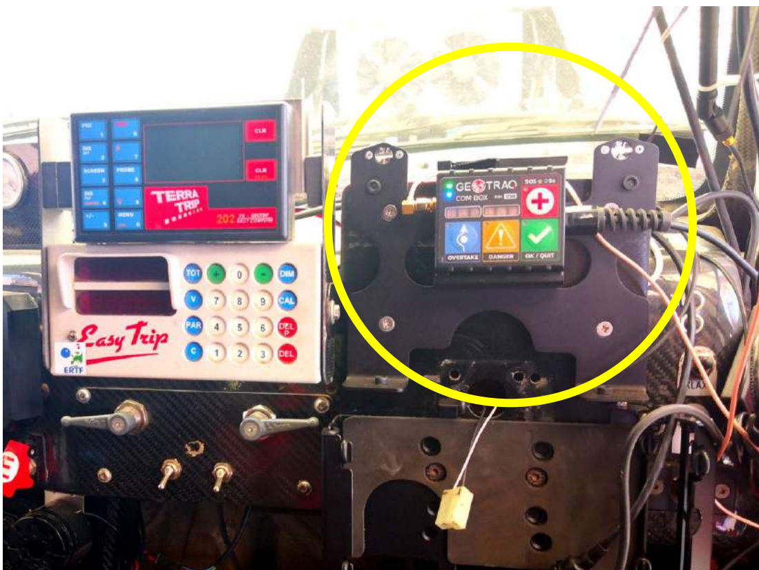
Installation of the Com-Box unit with bracket on the dashboard using bolts.
