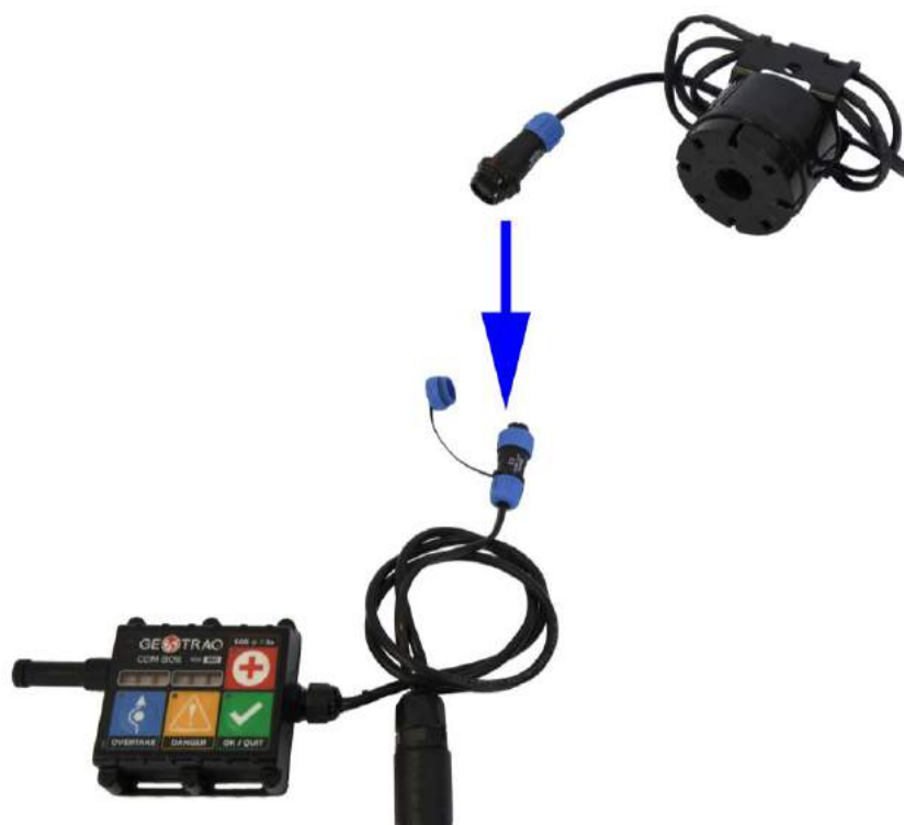
Connect the BUZZER to the COM-BOX.
