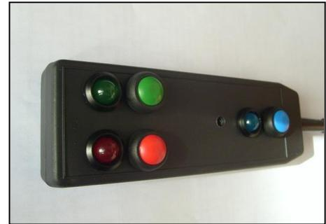
In case of stopping the car on the SS system is sending the warning signal to the car unit. The lamps in manipulator panel (Green and Red) start blinking. That means that operator of RCC see the car standing on the SS and expect to have the information from the crew. Within 1 minute from stopping over the Special Stage the driver or the pilot should press the proper button to clarify the situation.
