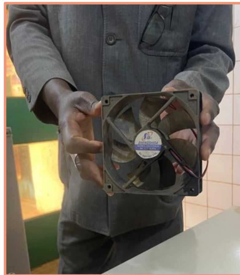
Cold chain technician in Tahoua showing the fan that is the part that breaks frequently on the fridges.
